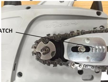
5. Fit the chain onto the drive sprocket and guide bar, so the fastening bolt and two guide fins fit into the keyway of the guide bar.
